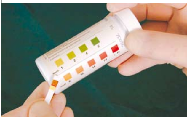
Figure 50. Compare the colour of the test strip with the colour scale on the container
